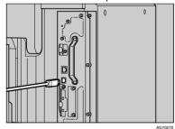
If the gigabit ethernet board is attached, connect the square-shaped connector of the USB2.0 cable to the USB port of the board.
