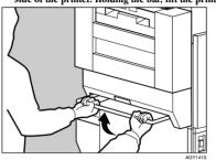
Remove the adhesive tape from the printer body. Remove the cardboard taped to the standard tray.
